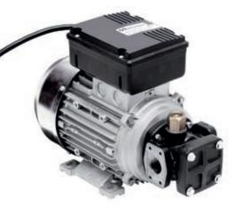
Internal gear electric pumps for lubricants. 230 V - 50 Hz (single-phase) or 380 V - 50 Hz (three-phase) motor, depending on model, IP-55 protection and on/off switch. Cast iron pump body, sintered steel gears and by-pass valve. Motor with mounting feet, the pump can be mounted horizontally on a flat surface or vertically on a wall.
