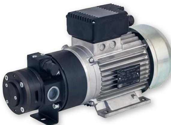
Electric gear pump, self-priming, for the supply of oil under demanding conditions at medium pressure and with long pumping distances; guarantees a constant flow and delivery, even after long pumping distances or with simultaneous supplies.
